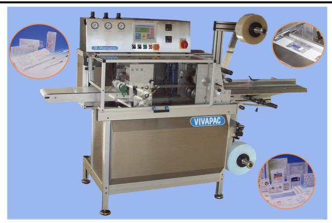
Horizontal Form Fill Seal machine, specially designed for automatic pouching of flat items in four side seals pouches. This user-friendly machine features simple and fast changeovers.
