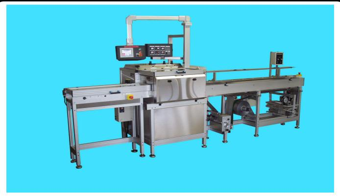
Horizontal Form Fill Seal machine, specially designed for automatic pouching of flat items in four side seals pouches from 2 rolls of thermosealable materials. All elements are driven by servomotors. Tactile screen interface with operator.
